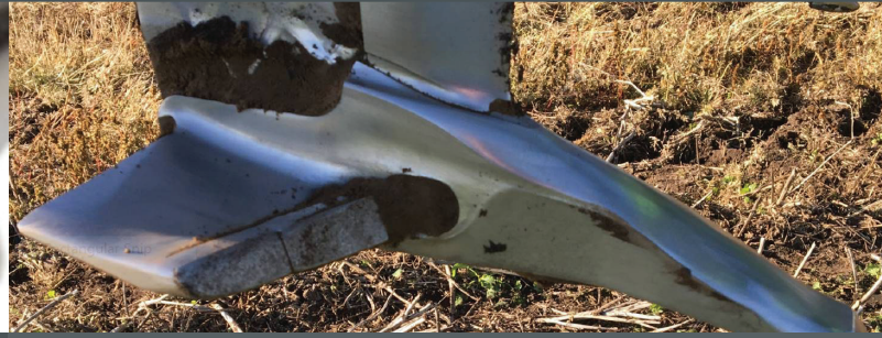
After 800 acres, the Ferobide reinforcement on this subsoiler foot still has a long way to go
