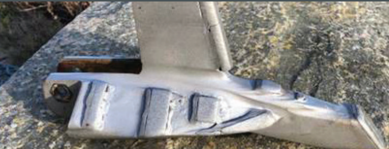
Sumo Subsoiler. 90 acres in very abrasive UK soils & 20mm Hardox™ leg is worn out. 470 acres in the same soils through strategic Ferobide placement.
