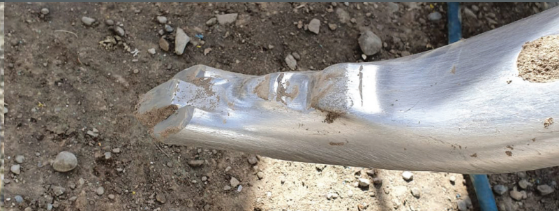
2 Ferobide tiles of 4 mm thickness placed behind original tungsten on a Vaderstad Topdown™.
