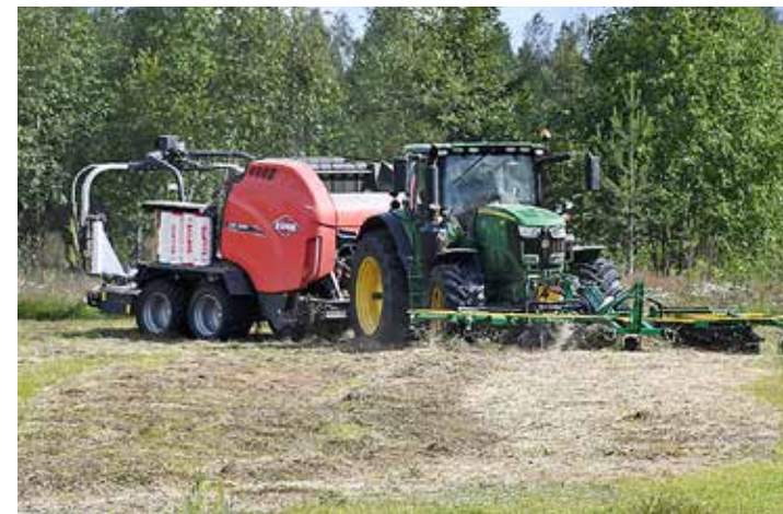
← When attached to the front linkage, the rake is slightly closer to the tractor than when attached to the front loader. To ensure free movement, there is a chain between the adapter and the frame instead of a topline.
