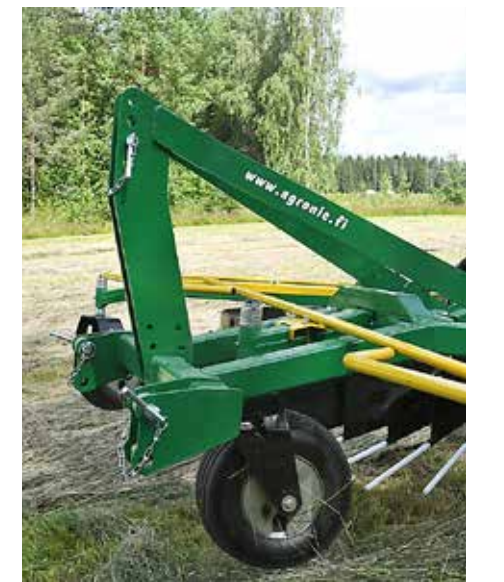
← When attached to the front linkage, the rake is slightly closer to the tractor than when attached to the front loader. To ensure free movement, there is a chain between the adapter and the frame instead of a topline.
