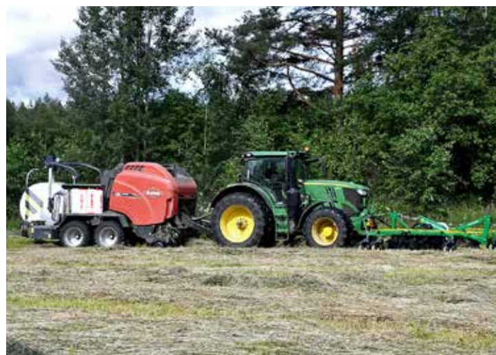
↑ Raking and baling is a single pass works successfully. Baling does not slow down while raking.
