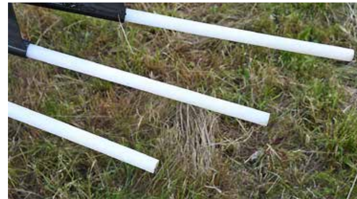
↑ Polyamide tines collect the hay, but usually leave the stones on the ground. Dirt contamination is minimal, even when the tine encounters the ground.
