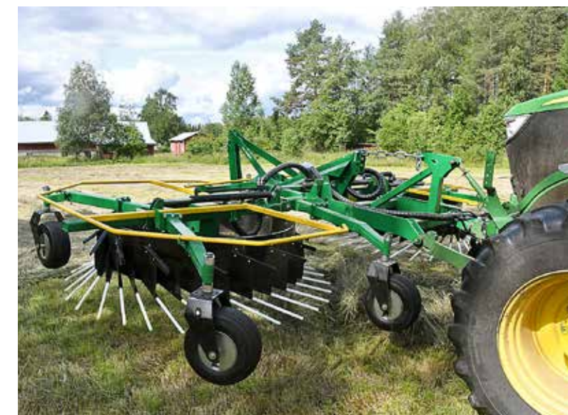
← When attached to the front linkage, the rake is slightly closer to the tractor than when attached to the front loader. To ensure free movement, there is a chain between the adapter and the frame instead of a topline.
